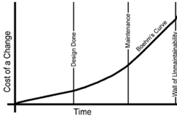
Figure 1-6: Cost of change over project lifetime [4]
